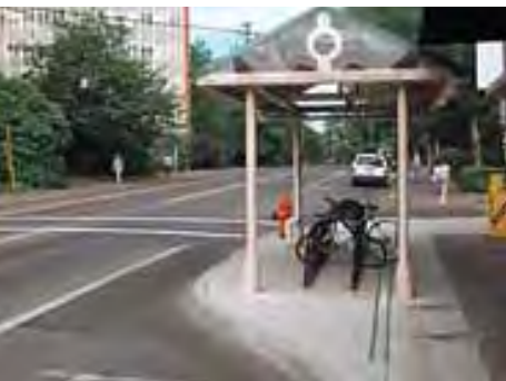
Curb Extension with Bicycle Parking
